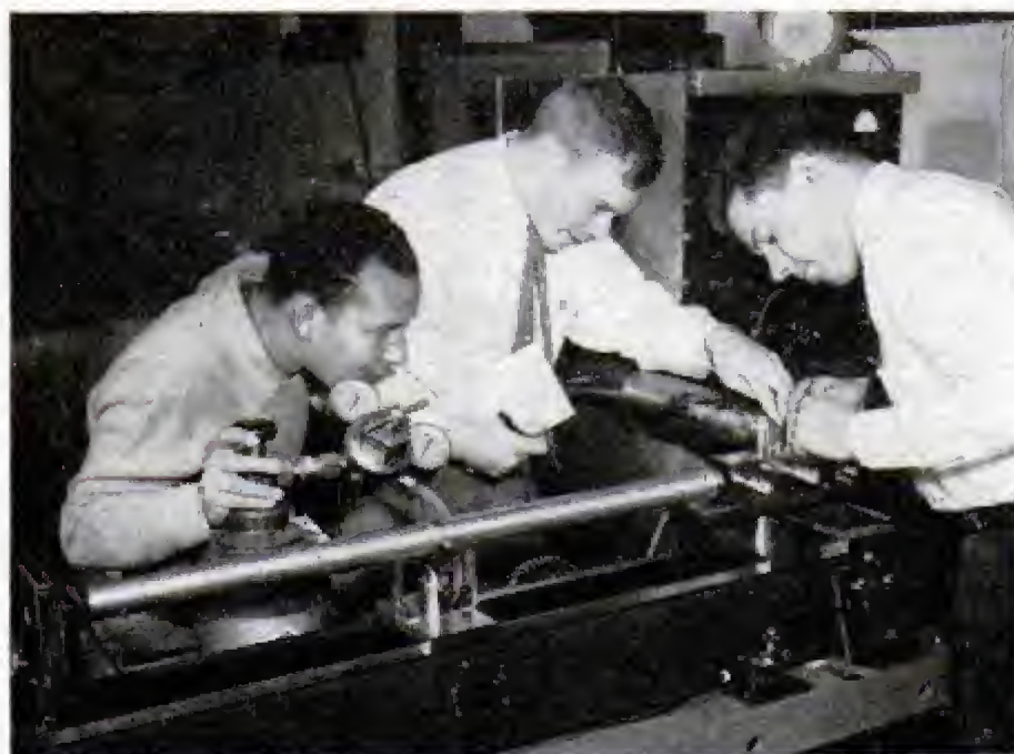
Specimen is placed in microscope. X rays pass through tube to film, left
